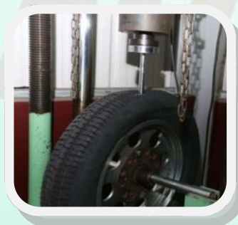
Breaking Energy (Plunger Test; Tire Strength)
