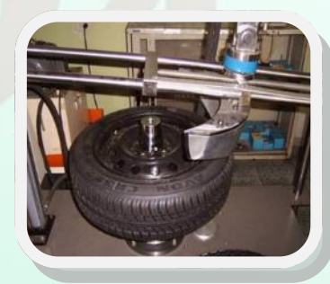
Bead Unseating Resistance Test
