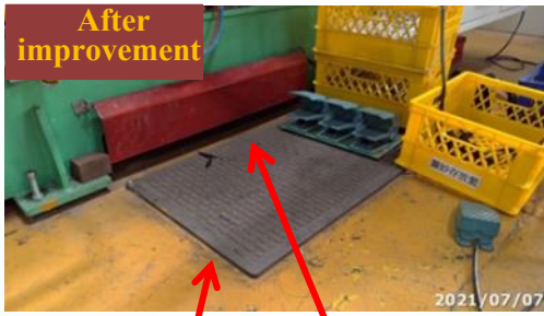
Description : Safety pad and emergency stop ladder board
